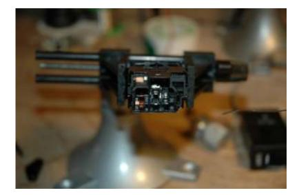
Above is the rear view of the STi Auto/Man switch without wiring for the DCCDPro controller in place.
