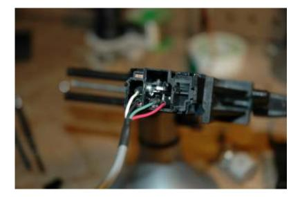
Above is the rear view of the STi Auto/Man switch with wiring for the DCCDPro controller in place.
